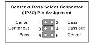
The 4 pin block jumper can be set to 1,2,3,4 or 3,4,5,6. The position this jumper block should be set to depends on your speakers. If during usage you find that your center and base channels are swapped set this jumper to the other position.
